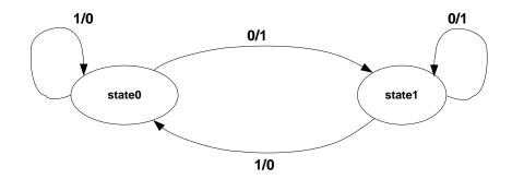
Finite state machines in VHDL can be implemented by following a typical programming structure such as given below. It consists of two processes: one for combinational logic process that sets the next state and output, and a clock handling process that loads the next state to present state. This implementation is a Mealy machine.
